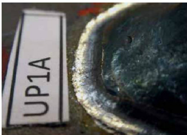
A weld toe treated with LETS Ultrasonic Peening Procedure
