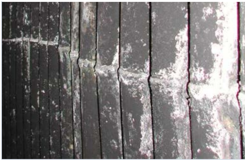
Figure 3. Mass deflection of gas-proof panel waterwall tubes in the field welded joints area detected on boiler No. 4 of "Dora" TPS (Iraq).
