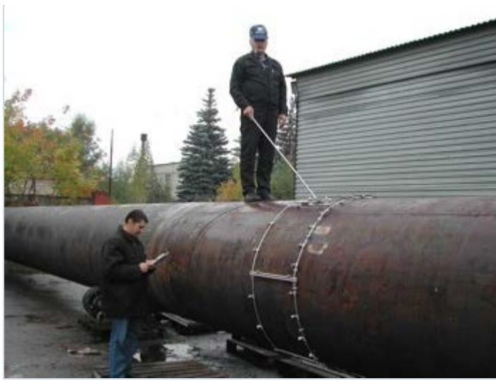
Fig.1. General view of the scanning device covering the entire diameter of a 1420 mm pipe with application of the instrument-computer complex based on the metal magnetic memory method.
