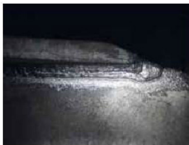
Bracket treated with LETS Global Ultrasonic Peening Procedure
