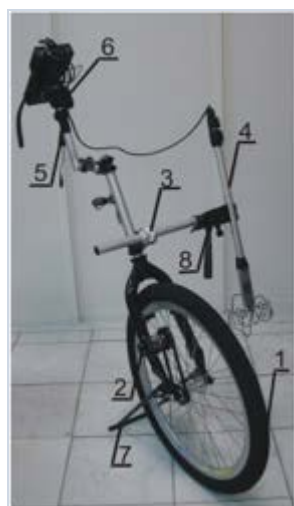
Figure 1. Appearance of the scanning device: 1 - road wheel; 2 - length-counting unit; 3 - Type 11 sensor attachment unit; 4 - Type 11 sensor; 5 - handle; 6 - measuring instrument mounting unit; 7 - folding support leg; 8 - universal head.
