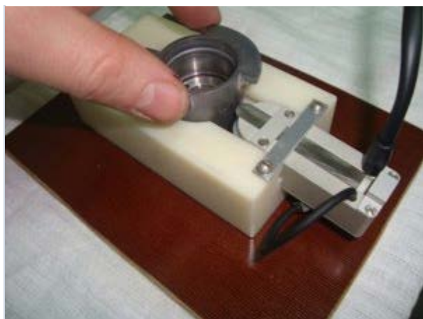
Figure 6. Scheme of a restrictor inspection using a SD integrated in a special device.
