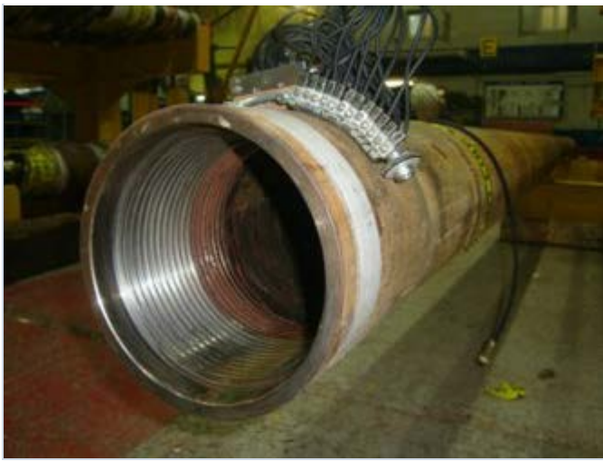
Figure 1. Borehole section (pump stator), female thread end view. SD (scanning device) is connected to the TSC type instrument.
